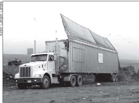
Litter abatement was enhanced through the Keller Canyon EIR. Now transfer trucks utilize an automated tarping system to prevent litter from leaving the trailer prior to disposal at the landfill.
